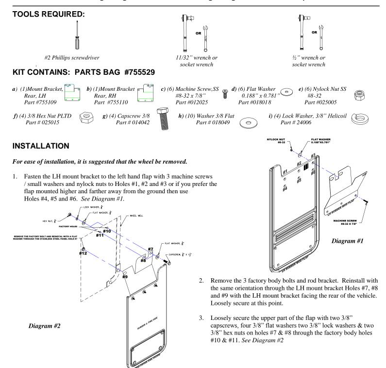
✓ Check all fasteners for tightness. Repeat procedure on the passenger side.
