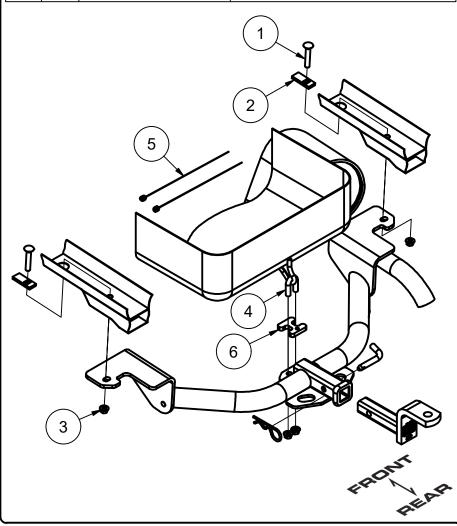
1) Lower the exhaust by removing the (2) rubber isolators from the hangers.
