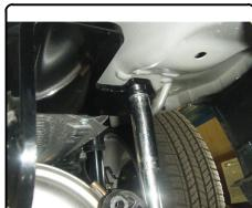
7) Raise the exhaust back into position and reintall the rubber isolators.
