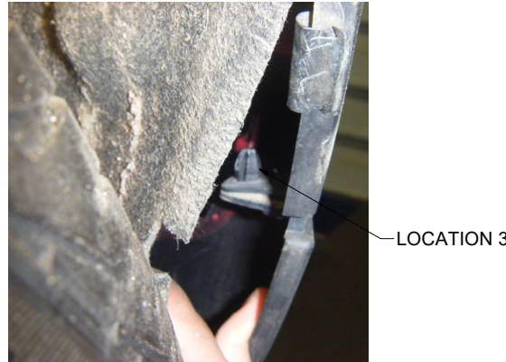
Photo 3: Fastener B behind rear wheel well liner.
