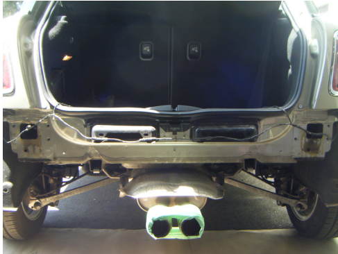
Photo 7: Bumper beam removed.
