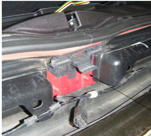
Photo 5: Tab located at center of hatch under the bumper cover.
