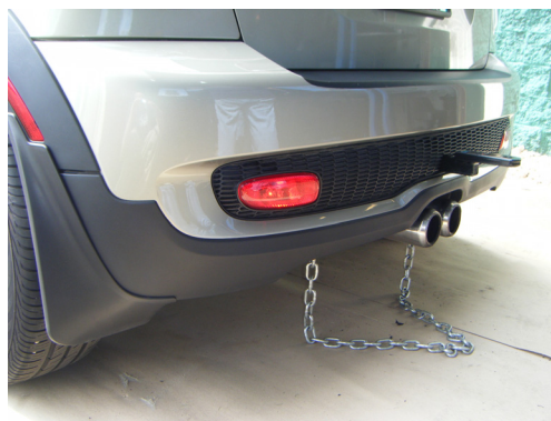
Photo 13: Hitch shown installed with safety chains
