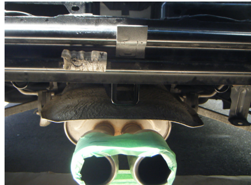
Photo 8: Hitch in position.
