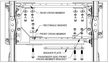
Figure B6: Bottom of truck frame looking up from the back of truck towards the cab
