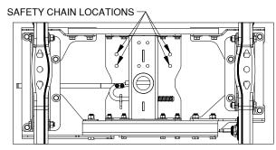
Figure F1: Bottom of truck bed looking up at hitch installation.
