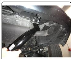
4. Torque all M12 hardware to 86 ft-lbs. Reinstall underbody panel removed in Step (1).
