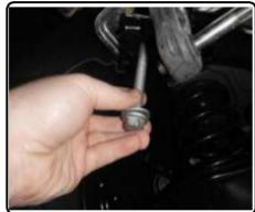
2. Reverse fishwire 1/2"-13 x 1 1/2" carriage bolts and CM-SP17 spacers into driver and passenger side frame rails.
