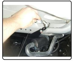
FISHWIRE TECHNIQUE INSERT COILED END OF FISHWIRE TOOL THROUGH HITCH MOUNTING HOLE IN VEHICLE FRAME RAIL AND OUT THE ACCESS HOLE. PASS COILED END OF FISHWIRE THROUGH SPACER AND THREAD BOLT INTO COIL KINK WIRE TO KEEP SPACER SEPARATE FROM BOLT AS SHOWN. PULL CCES ISHWIRE, SPACER, AND BOLT THROUGH FRAME AND OUT MOUNTING HOLI JSE FISHWIRE TO GUIDE HITCH DURING MOUNTING AND PREVENT LOSS OF BOLT PACER INSIDE FRAME RAIL. \*\*NOTE: SOME VEHICLES MAY FISHWIRE THROUGH END OF FRAME
