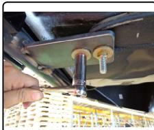
4. Loosely secure the (4) M10 bolts supplied into weldnuts in the vehicle frame. (Weld nut cleaning with a wire brush or lubricant maybe required).
