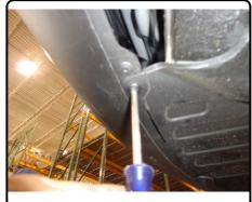
2. Lower exhaust by disconnecting the rubber isolator from the exhaust hanger.
