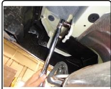
6. Raise exhaust into original position. Install complete.
