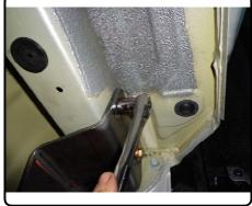
5. First torque the 3/8" U-bolt to 30 lb-ft and then the M10 bolts to 51 lb-ft.
