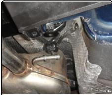
2. Remove the (4) lowest M8 bolts from the bumper beam and return to vehicle owner.
