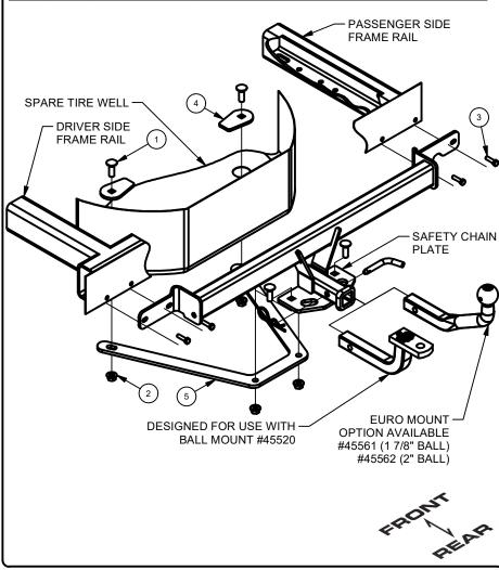
1. Remove (3) torx head bumper cover retention screws. Temporarily lower the exhaust by removing the rubber exhaust isolator. (Save screws for use in Step 4)
