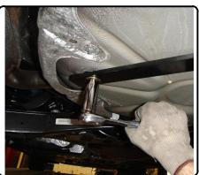
8. Return spare tire and other items removed in Step 8 to the trunk. Torque 1/2" fasteners to 110 ft-lbs and M8 fasteners to 23 ft-lbs.
