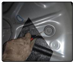
6. Use silicone caulk (or equivalent) to seal the tire well plug hole from exhaust fumes and water by putting a bead around each hole inside the spare tire well. Place a 11410-SP spacer onto each hole and put a bead of caulk around each square hole. Install a 1/2" carriage bolt into each hole.
