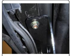
7. Using a 3/4" socket, torque 1/2" hardware to 110 lb-ft. Using a 17mm socket, torque M10-1.50 hardware to 56 lb-ft. Reinstall the (2) bumper cover fasteners removed in step 1.
