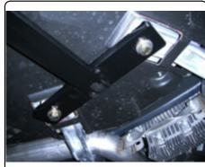
5. Press hitch against the bottom of the bumper beam, with the hitch centered, using the hitch as a template mark hole locations with a center punch. Lower hitch and drill hole locations with 17/32" drill bit.
