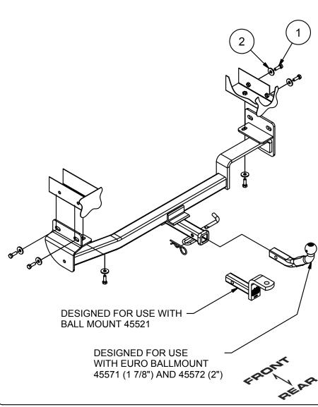
Note: Be careful around the brake lines and the canister.
