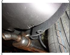
2. Lower exhaust by removing rubber exhaust hangers from hanger rods in (1) location on the passenger side.
