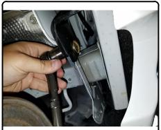
4. On the underbody panel, mark out a 2.375" x 2.25" section centered on the panel using masking tape and trim using aviation shears. Trim off the driver side of the panel from the far most clip using aviation shears. Reinstall following Step 1 in reverse order. **NOTE**: The dimensions are approximate. Confirm fit prior to install.
