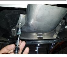
To lower exhaust, remove (2) bolts using an E12 socket from the exhaust bracket on each side. Locate and remove (2) rubber isolators from the exhaust towards the front of the vehicle.
