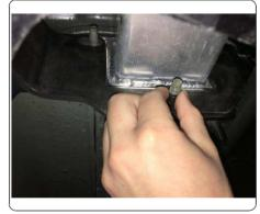
5. Use 15mm socket and torque all vehicle hardware to 45 ft-lbs. Reinstall hardware removed in step 1.
