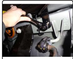
6) Torque all 7/16" hardware to 59 lb-ft. Torque all M12-1.25 hardware to 86 lb-ft. Torque all M12-1.75 hardware to 79 lb-ft. Raise exhaust hangers back into position.
