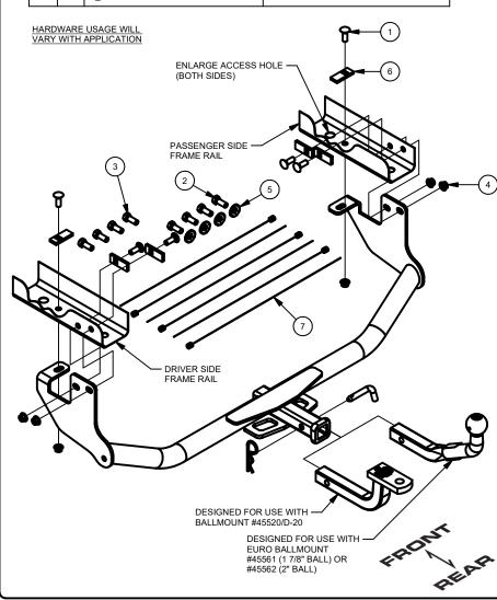
1) Lower rear exhaust hangers from one location on each side of the vehicle. For ease of installation, the exhaust can also be lowered in one location at the front center of the vehicle. This location will need to be lowered slowly and supported from underneath during install. Caulking may need to be trimmed around side mounting holes if present.
