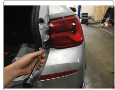
6. Remove rear fascia by locating and removing fastener behind tail light cover using 8mm socket and unclip rear fascia attachments.
