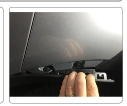
Open rear hatch to expose and remove plastic cover located inbore of each tail light, remove (1) fastener on each side flathead screwdriver.
