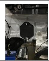
8. Raise hitch into position using studs to align. Reinstall rear bumper beam over hitch and secure using existing vehicle hardware.
