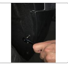
2. Remove (3) rivets along wheel well trim above each rear tire using a small punch and pry tool.
