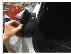
5. Remove (2) bolts from each tail light using 10mm socket. Carefully remove tail light from vehicle and unclip electrical harness.
