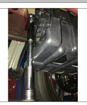
2. On passenger side lower exhaust by removing (2) exhaust isolators, using isolator removal diagram, to expose heat shield. Remove (4) speed nuts to lower heatshield from frame rail.
