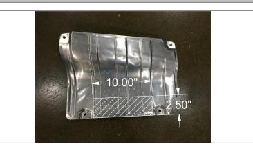
4. Enlarge forward most attachment hole on both sides using a die grinder. Use hole enlargement diagram as a reference.
