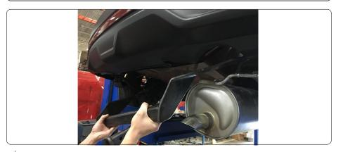
8. Torque all 7/16 hardware to 59 ft-lbs. Reinstall emmisions canister, raise exhaust into position.
