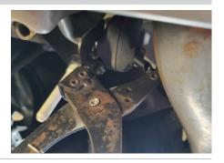
Remove the electrical harness from the frame rail. Move electrical harness from under the bumper beam to above the bumper beam.
