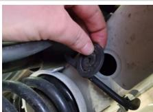
Fishwire three 7/16" carriage bolts (#1) and three spacers (#3) from the holes where the rubber plug was removed in step 3 to each of the three holes in the frame rail. Repeat on the other side of the vehicle.
