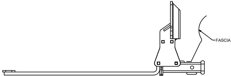
INSTALLED HITCH POSITION
