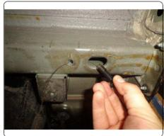
5. Reverse fishwire 1/2" carriage bolts and SP10 spacers through the access hole. Carefully pull bumper cover and raise hitch into position. Loosely fasten the hitch using 1/2" flange nuts on both sides.
