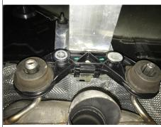
Remove heat shield using needle nose pliers to loosen (4) speed nuts on driver side and (2) speed nuts on passenger. Trim heat shield using aviation shears as shown in Heat Shield Trim Diagram. Reinstall trimmed heat shield.
