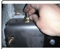
8. Torque all 1/2" fasteners to 110 lb-ft. Torque all M14 fasteners to 126 lb-ft. Torque all M8 fasteners to 23 lb-ft.
