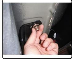
5. Torque all 12mm hardware to 86 lb-ft and all 7/16" hardware to 59 lb-ft. Reinstall exhaust deflector.
