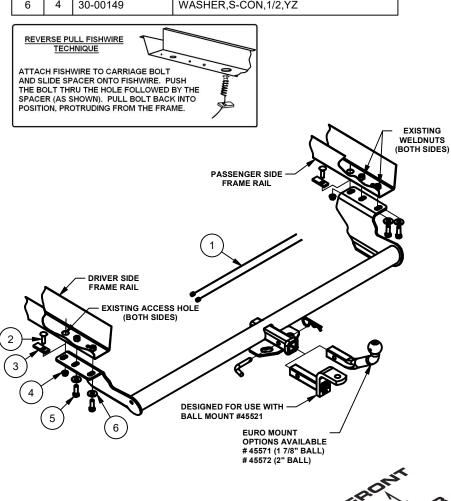
1. If present, remove (6) fasteners ((4) plastic push pins, (1) phillips head screw and (1) hex bolt with 10mm socket) and the plastic underbody panel covering the driver side frame rail. Return fasteners and plastic shield to owner. Remove (2) fasteners on the exhaust deflector and temporarily remove deflector.
