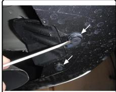
2. Reverse fishwire (2) 7/16-14 x 1 1/2" carriage bolts and CM-SP2 spacers into the existing hole in the bottom of the frame rails leaving the fishwires attached.
