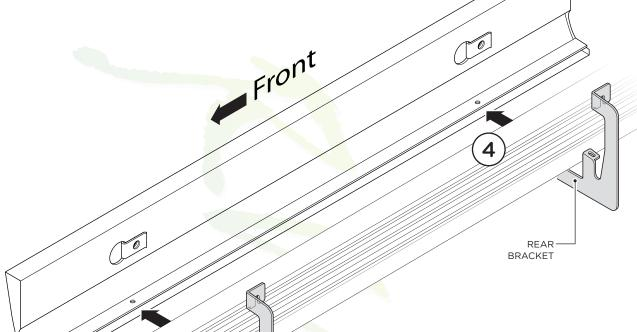
**5.** Fasten lower portion of the Front Bracket using one (1) M8 x 30MM Hex Head Bolt, one (1) M8 Lock Washer, one (1) M 8 Flat Washer, one (1) Weld Support and one (1) M8 Flange Lock Nut. Repeat for Rear Bracket.
