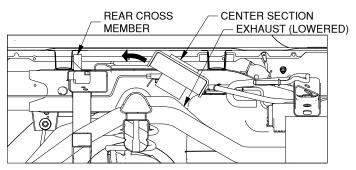
Figure C2: Cut-away view looking towards the inside of the driver side frame.
