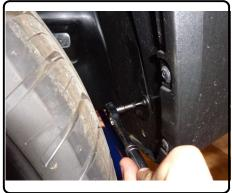
4. Fishwire (2) 1/2" carriage bolts and (2) CM-SP10's into the holes on the outside of each frame rail. Reverse Fishwire (1) 1/2" carriage bolt and (1) CM-SP10 into the hole on the bottom of each frame rail. Keep fishwires attached until hitch is raised into position.
