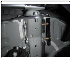
4. Raise hitch into position and slide the bolts through to support it. Loosely install the supplied hex flange nuts and the (2) hex bolts and conical washers as shown. Be sure teeth on washers are against the hitch mounting plate.
