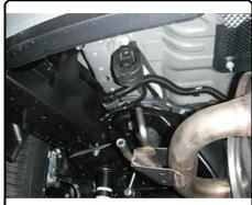
2. If present, remove the tow loop on the passenger side of the vehicle frame. Return tow loop and bolts to vehicle owner.
