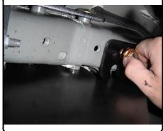
5. Torque all 10mm fasteners to 48 lb-ft and all 1/2" fasteners to 110 lb-ft.
