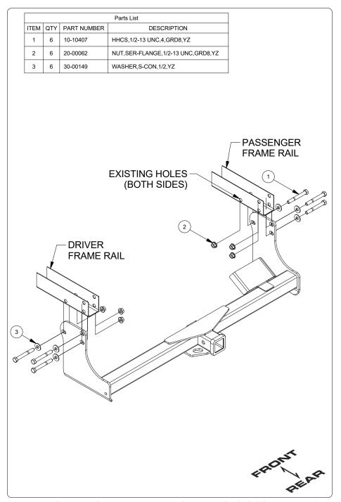
1. Locate tie-down loop on passenger frame rail and remove (2) M10 bolts on the bottom of the frame using a 16mm socket. Remove (2) M12 bolts on the inside of the frame using an 18mm socket and 18mm wrench. Return tie-down loop to owner.
