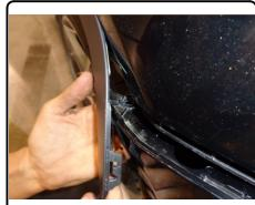
Remove heat shield by removing (10) nuts using 8mm socket, and trim 2.00" x 3.00 " using avaition shears as shown in the trim diagram. Set aside for reinstallation.
