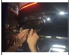
2. Lower exhaust by removing (3) rubber isolators. (As shown in the rubber isolator removal diagram)
