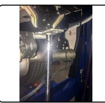
Install hitch on rear of vehicle frame using exisiting studs.
