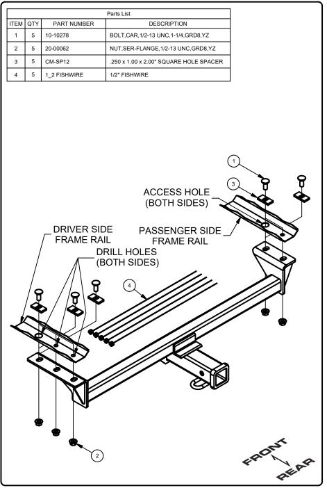
1. Lower the exhaust by removing the (2) rearmost rubber exhaust isolaters from the frame mounted hangers. Be sure to support the exhaust during installation to prevent damage.
