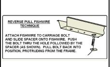
8. Raise hitch into postion running the fishwires through the holes on the hitch. Remove fishwires and loosely fasten (5) 1/2" flange nuts.
