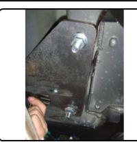
10. Install rubber isolators removed in Step 1 onto muffler hangers in side plates on each side. Raise exhaust into position and reinstall muffler hangers in rubber isolators.
