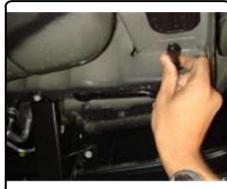
Located on driver side frame rail, fishwire (1) CM-SP10 spacer and (1) 1/2" carriage bolt through access hole and out mounting hole.
