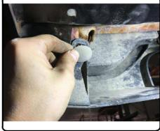
9. Torque 1/2" hardware to 110 ft-lbs, torque M12 hardware to 79 ft-lbs and 7/16" hardware to 59 ft-lbs
