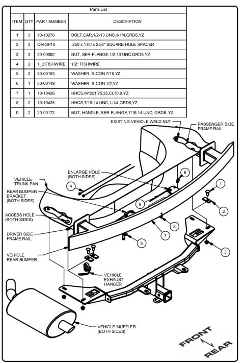
Lower exhaust by removing (2) exhaust hanger brackets from rubber (1) isolator on each frame rail.
