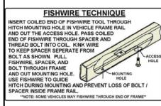
Reverse fishwire (1) CM-SP10 spacer and (1) 1/2" carriage bolt through and out access hole on each frame rail. (As shown in Reverse Fishwire Technique Diagram)
