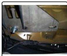
8. Located on rear bumper bracket insert 7/16" handle nut through opening, hand tighten 7/16" hex bolt through enlarged hole with conical tooth washer.
