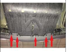
2. Fishwire (2) 7/16" carriage bolts and (2) CM-SP2 spacers through the vehicle access holes to the attachment holes on each side. See FISHWIRE DIAGRAM below.
