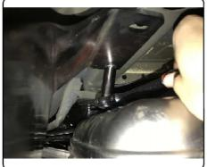
5. Torque all 7/16" hardware to 59 ft-lbs and all 1/2" hardware to 110 ft-lbs. Reinstall items removed in Steps 1.
