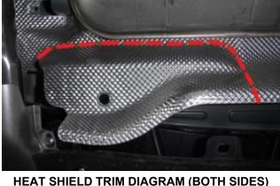
HEAT SHIELD TRIM DIAGRAM (BOTH SIDES)
