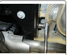
8. Remove the clip nuts from the (3) bumper brackets removed in step 1 and install onto the tabs on the Main Body Weldment. Align the clips with the lower bumper fascia tabs and reinstall the (4) screws removed in step 1.
