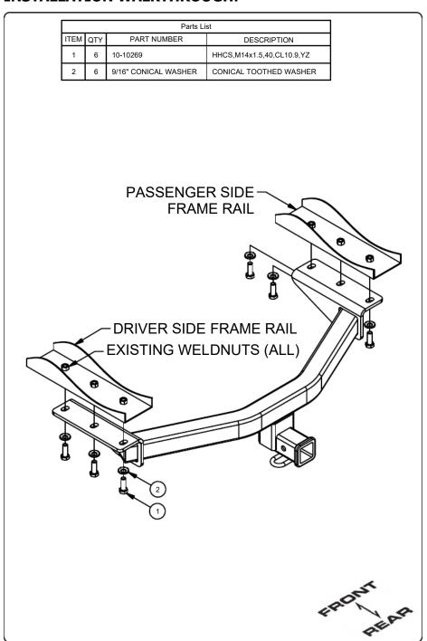
Raise hitch into position and secure with the provided M14 bolts and 9/16" conical washers.
