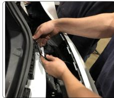
5. Locate and remove (5) fasteners from rear plastic trim using a 10mm socket. To remove bumper beam locate and remove (6) nuts, (3) on each side, using 15mm socket. Set aside hardware and bumper beam for reinstallation. To remove bumper beam plates remove (8) nuts, (4) on each side using 15mm socket. Return bumper beam plates to owner.
