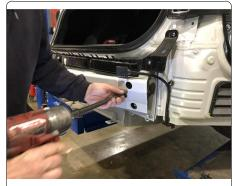
6. Use 7/16 hardware to assemble rear bumper and hitch. Raise assembly into position using vehicle studs to align on rear of vehicle. Use hardware removed in Step 5 to secure hitch to vehicle. Torque M10 hardware to 45 ft-lbs. **NOTE:** Use nylon washers to avoid hitch-vehicle contact.
