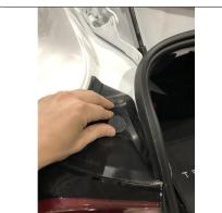
2. To remove tailight locate and remove (2) nuts, on each side, using 8mm socket. Unplug electrical harness and gently remove tailight. Set aside tailight for reinstallation. Remove exposed fascia screw using 10mm socket, on each side.
