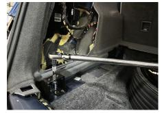
For Audi Q5 with bumper fascia hitch access panel: Using a T25 socket, remove (2) torx screws and remove hitch access panel from bumper fascia. Return access panel to owner.
