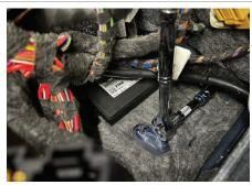
Using a T-25 socket, remove four (4) torx screws per side from the driver- and passenger-side wheel well liners.
