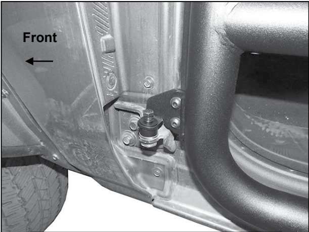
(Fig 16) Tighten hardware on Hinges (driver/left Lower Hinge pictured)
