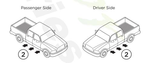
**3.** Remove the **Tape** covering the factory oblong hole in the rocker panel located above the two (2) hex holes.
