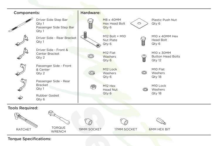
For Rocker Panel Mount Installations M8 through M12 bolts and nuts are set to 15-20 ft lbs.
