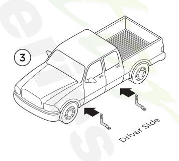
**4.** Align the Front and Rear Driver's Side Brackets with existing bolts located on the rocker panel of the vehicle.
