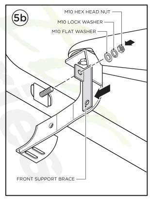
**6.** Fasten the Front Support Brace to the Front Bracket using one (1) M10 Lock Washer, two (2) M10 Flat Washers, one (1) M10 Hex Head Nut and one (1) M10 x 30MM Hex Head Bolt.
