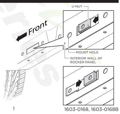
**4.** Install the Top Flange of the Passenger Side Front Bracket by fastening two (2) M10 X 30MM Hex Head Bolts, two (2) M10 Flat Washers and two (2) M10 Lock Washers into the M10 U Nut Clips.
