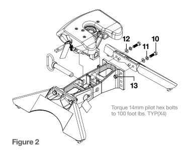
**NOTE:** The head assembly can easily be removed from the midsection to further aid installation of the hardware.
