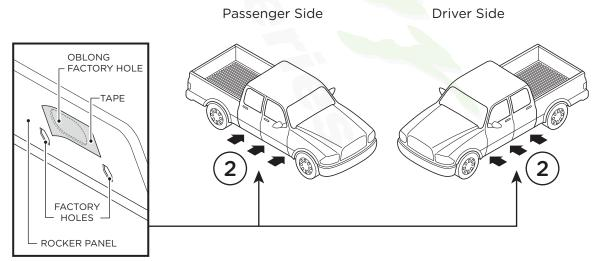
**3.** Begin installation on passenger side. Position Front Bracket, Center Bracket and Rear Bracket as shown along passenger side.
