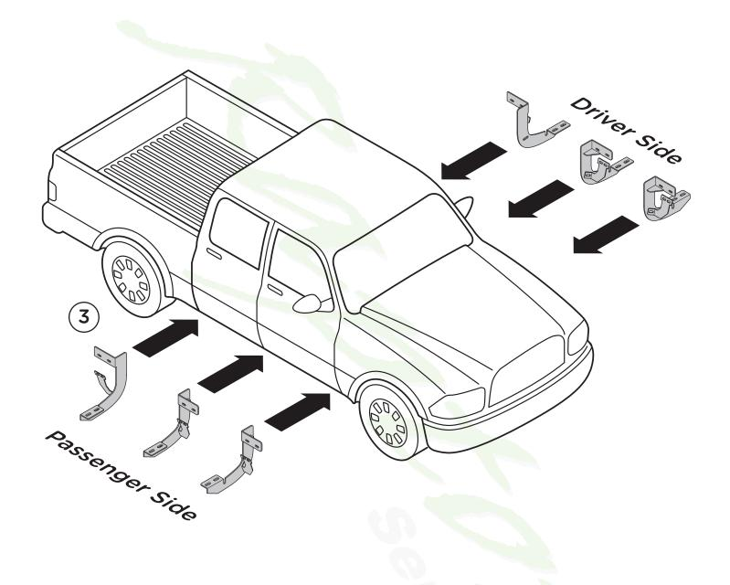
**4.** If threaded inserts already exist in Rocker Panel holes, fasten the top portion of the bracket by using (2) M8 x 30MM Head Head Bolts, (2) M8 Flat Washers and (2) M8 Lock Washers.
