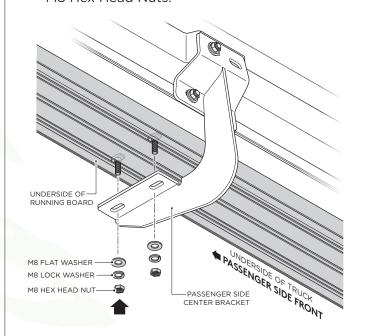
**11.** Fasten the Running Board to the Passenger Side Rear Bracket cradle by using (2) M8 Flat Washers, (2) M8 Lock Washers and (2) M8 Hex Head Nuts.
