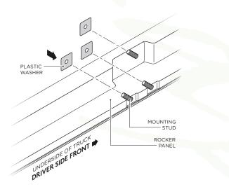
**4.** Fasten the top portion of the Driver Side Front Bracket by using (2) M8 x 30MM Hex Head Nuts, (2) M8 Flat Washers and (2) M8 Lock Washers.
