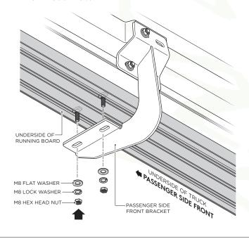
**10.** Fasten the Running Board to the first Passenger Side Center Bracket cradle by using (2) M8 Flat Washers, (2) M8 Lock Washers and (2) M8 Hex Head Nuts.
