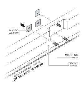
**6.** Fasten the top portion of the Driver Side Center Bracket by using (2) M8 x 30MM Hex Head Nuts, (2) M8 Flat Washers and (2) M8 Lock Washers.
