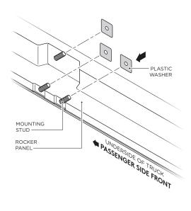
**6.** Fasten the top portion of the Passenger Side Center Bracket by using (2) M8 x 30MM Hex Head Nuts, (2) M8 Flat Washers and (2) M8 Lock Washers.
