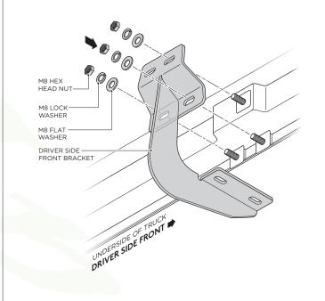
5. Locate the three existing Mounting Studs located on the interior wall of the Rocker Panel. Place Plastic Washers onto each Mounting Stud to prevent corrosion caused by aluminum to steel contact.
