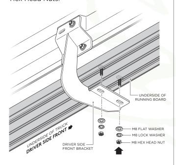
**10.** Fasten the Running Board to the first Driver Side Center Bracket cradle by using (2) M8 Flat Washers, (2) M8 Lock Washers and (2) M8 Hex Head Nuts.
