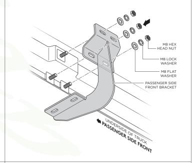
**5.** Locate the three existing Mounting Studs located on the interior wall of the Rocker Panel. Place Plastic Washers onto each Mounting Stud to prevent corrosion caused by aluminum to steel contact.
