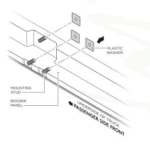
**4.** Fasten the top portion of the Passenger Side Front Bracket by using (2) M8 x 30MM Hex Head Nuts, (2) M8 Flat Washers and (2) M8 Lock Washers.
