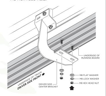
**11.** Fasten the Running Board to the Driver Side Rear Bracket cradle by using (2) M8 Flat Washers, (2) M8 Lock Washers and (2) M8 Hex Head Nuts.
