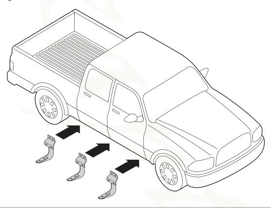
2. Passenger Side Front Bracket cradle (2a), Driver Side Center (2b) cradle and Rear Bracket cradle (2c) will face toward the front of the truck.
