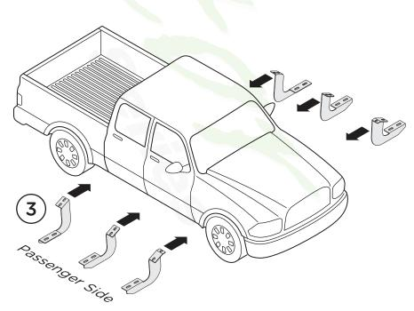
**4.** Install the first passenger side Bracket closest to the front wheel. Align with existing factory holes in the rocker panel as shown (4a), Secure the first Bracket using two (2) M8 x 30mm Hex Bolt, two (2) M8 Lock Washer and two (2) M8 Flat Washer (4b).
