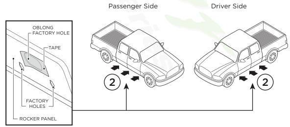
**3.** Begin installation on passenger side. Position Front Bracket, Center Bracket and Rear Bracket as shown along passenger side.
