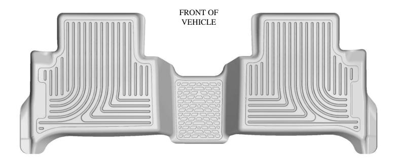
TO EASE INSTALLATION OF YOUR COLORADO / CANYON SECOND SEAT LINER, MOVE THE FRONT SEATS TO THEIR MOST FORWARD POSITIONS. WITH THIS DONE, INSERT LINER IN VEHICLE ANGLING THEM SO THAT THE FRONT EDGE OF THE LINER IS SEATED INTO PLACE FIRST, THEN LOWER THE REAR OF THE LINER. ONCE THE LINER IS INSTALLED, REPOSITION THE FRONT SEATS AS DESIRED.
