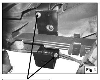
(Hook Plates) 12mm x 45mm Hex Bolts 12mm Lock Washers 12mm Flat Washers
