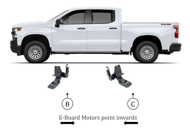
**Step 10**: Repeat Steps 2-6 to install the motor linkage assemblies. Repeat steps 8-9 to install running board on the Passenger side.
